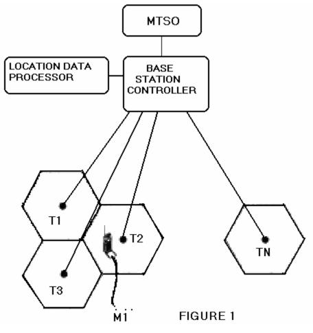
Configuration of a typical mobile telecommunication network.
