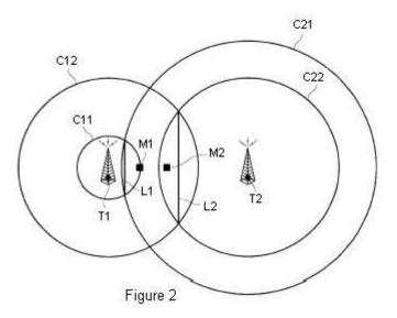
Figure 3.4, illustrates the TDOA method of locating a mobile telephone.
