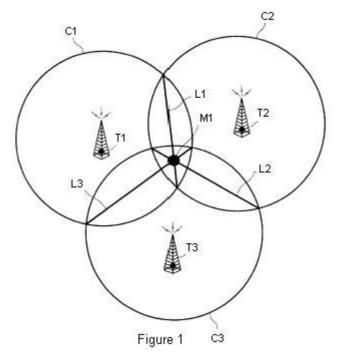
Figure 3.3 illustrates a typical TOA method for locating a mobile telephone.
