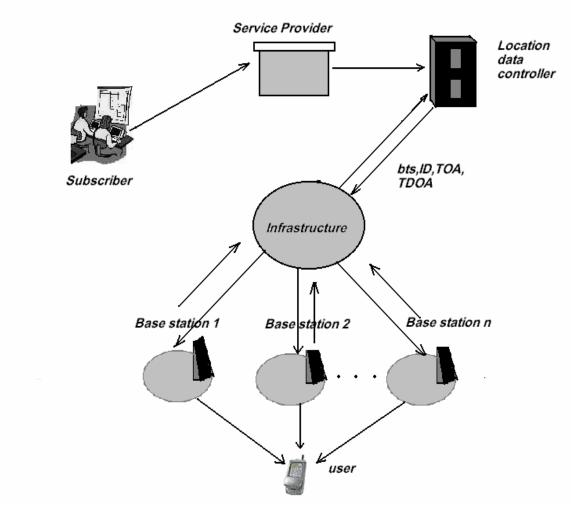
(Fig)2.1 Architecture of a general Geolocation system
