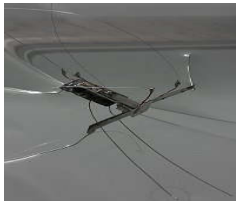
This robot has water-resistant legs to make Sure it floats in water
